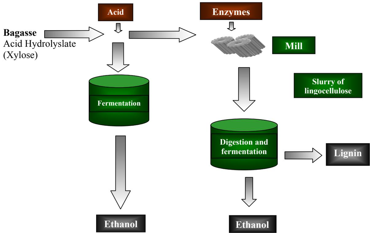
**Figure 5: Bagasse - to - ethanol process**
